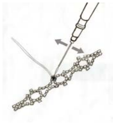
Soldering with a vibrating flame
