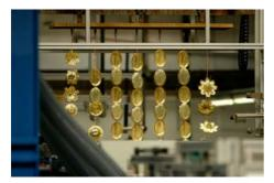
Electroplating is a plating process that uses direct current in order to deposit thin layers of the desired metals from a solution of their salts on electrically conductive objects.
